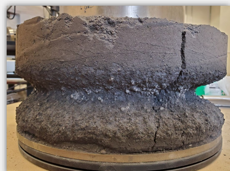
Figure 4. Spalled Nectar Simulant
